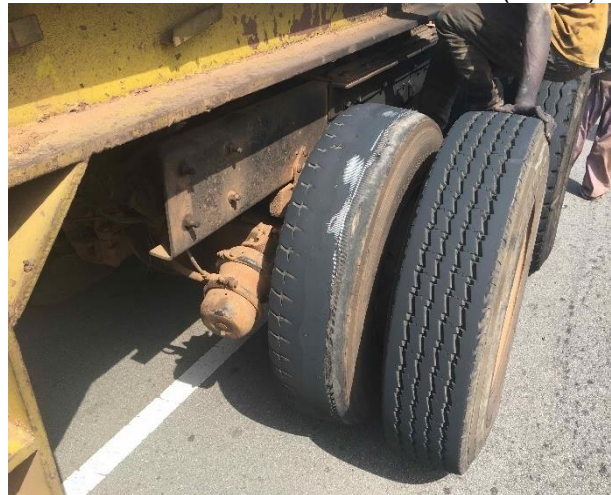
Figure 4.9 – Defective tyres in Liberia (Jan’18)
